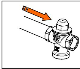
Mount the valve on the pipe, paying attention to the direction of flow shown by the "ARROW" on the body.
