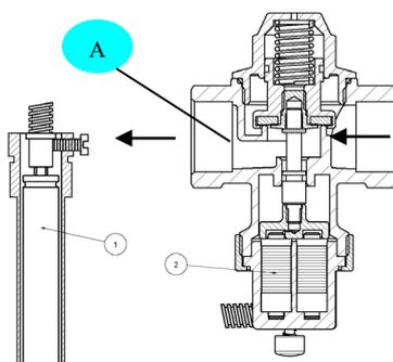
As the temperature of the water in the circuit increases, a liquid-gas phase change takes place inside the sensitive element (Point 1 in the figure), resulting in increased volume inside the capillaries and therefore dilatation of the bellows (Point 2), which press against the shutter and open passageway "A".
