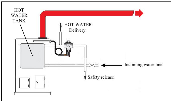
Example of safety release valve installed on a boiler with a built-in hot water tank.
