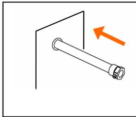
Mount the sensor holding trap on the upper part of the boiler or on the outgoing line, so that it comes before all on/off controls.
