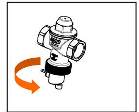
Turn the flexible sheath connecting up the probe by turning its cap. Now tighten the ring all the way.
