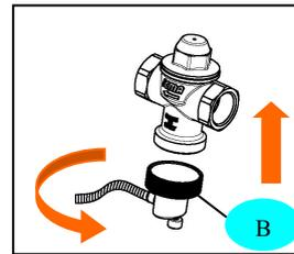
Put the sensor support cap in its housing, then tighten the textured ring (B) by hand.
