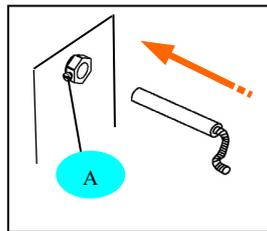
Insert the capillary in its trap, locking it with the screw (A).
