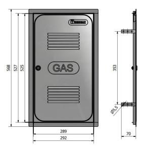
Gas meter door made of fibreglass with anti-UV treatment and anti-cut galvanised sheet metal frame; designed for gas metering units with a volumetric flow rate up to 6m<sup>3</sup>/h.
